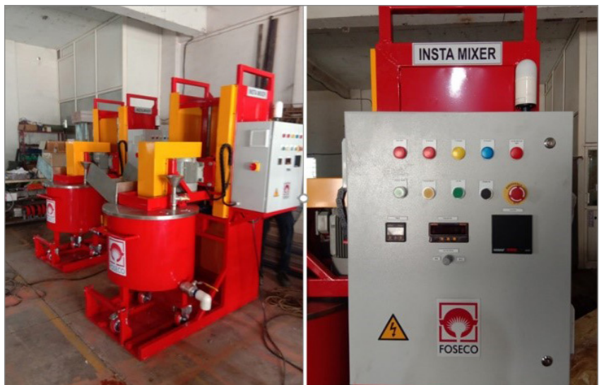
Figure 4. INSTA coating and Mixer for coating preparation at Bradken
