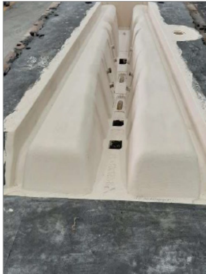
Figure 5a and b. Mould/core coated with INSTA coating
