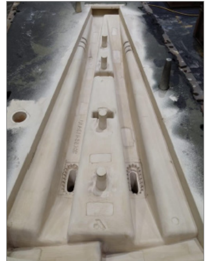
Figure 4a and b. Shows the mould/core before coating with INSTA coating.
