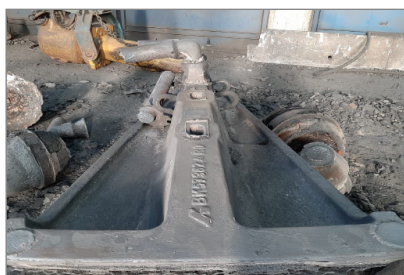
Figure 6a and b. Casting results with HOLCOTE INSTA
